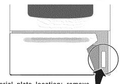
Serial plate location; remove lower panel (on some models) or storage drawer.
